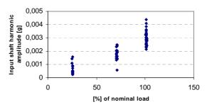
Fig. 2. Correlation between input shaft harmonic amplitude and load obtained for high power gearbox dedicated for conveyor drives
