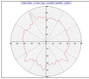
Fig. 10. AMF profile averaged over the rotation period of the geared roll (TMAeff=11%, TMApp=26%)
