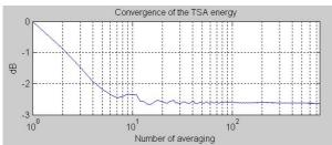
Fig. 2. Convergence of the TSA energy versus the number of averaging for the 24 tooth pinion
