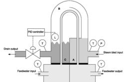
Fig. 1. Schem of a feedwater heater [5] (A: desuperheating area; B: condensing area; C: subcooling area; T: temperature sensor; L: level sensor; P: Pressure sensor)
