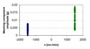
Fig. 3. Differences between meshing component amplitudes for different speed direction
